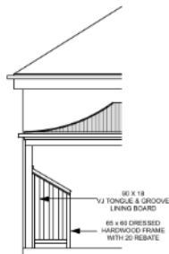
E ELEVATION TIMBER PANELING
